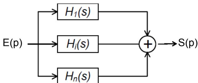
$$T(p) = \frac{S(p)}{E(p)} = H_1(p) + H_2(p) + \dots + H_n(p)$$
