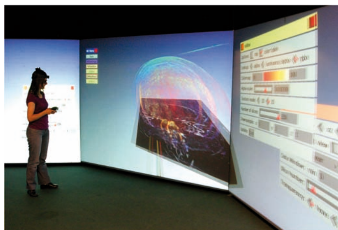
3-wall stereoscopic display environment with wireless tracking for immersive and interactive visualisation of medical data.
