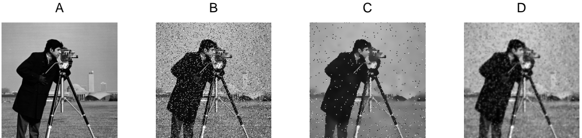
Fig. 2. Visual comparison of the performance of the restoration processes by Eq. (2) and Eq. (3). A : the original 'cameraman' image \psi_{ori} of Eq. (1). B : the noisy version \psi_0 of \psi_{ori} corrupted by an additive salt and pepper noise \xi (Eq. (1)) of standard deviation 0.1 ; C and D are respectively obtained with Eq. (2) and Eq. (3) for the optimal number of iteration n corresponding to the highest value of the normalized crosscovariance in Fig. 1 ( M = 11 in the case of D).
